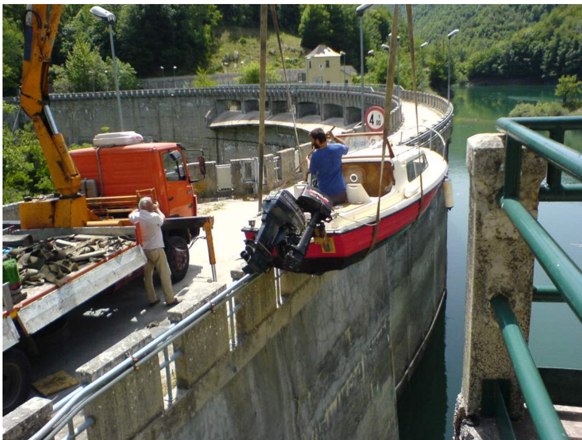
Vessel deployed by crane from dam wall.
